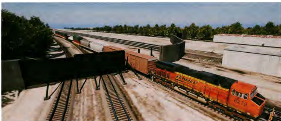
Rendering developed by HNTB of the 24' tall Santa Fe Junction stop log closure showing scenario of a partial stop log installation and live railroad traffic right before full closure. HNTB provided preliminary and final design of this BNSF crossing and is currently working with USACE in an oversight role as it is constructed.
